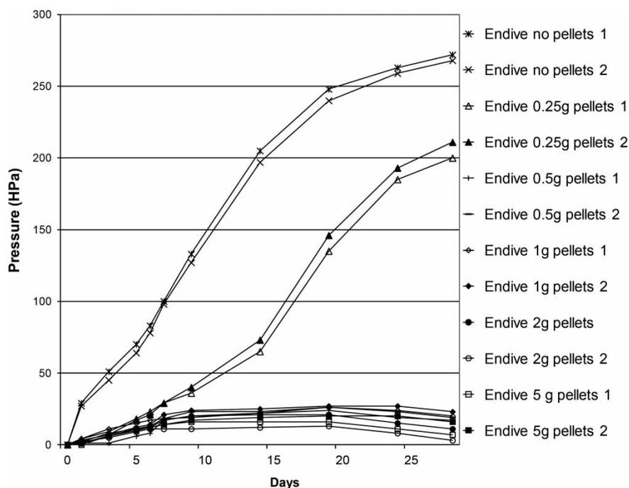
Figure 2 | Cumulative biogas production measured as pressure increase of samples treated with different amounts of NaOH pellets in the headspace.
