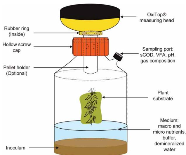
Figure 1 | Schematic representation of the batch set-up employed.
