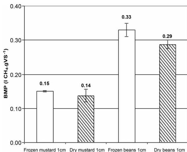
Figure 6 | Effect of drying samples at 65 °C in BMP results using mustard and green beans as substrates.
