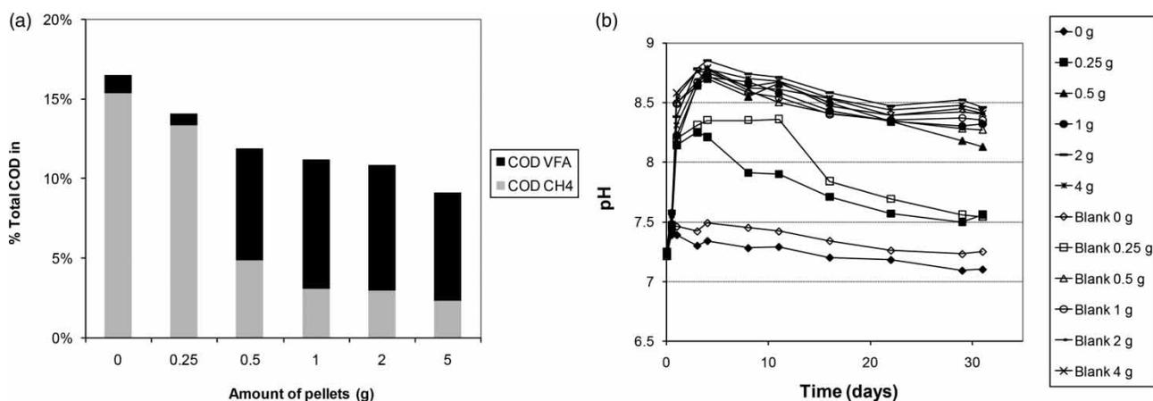
Figure 3 | Effect of NaOH pellets in COD conversion (a) and pH (b) during BMP assessment of frozen blended endive.
