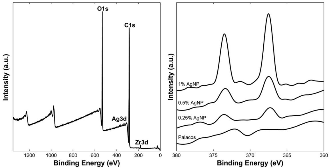
Fig. 5. XPS spectra of the cements. Left – XPS survey spectra, right – high-resolution XPS spectra of Ag3d.
