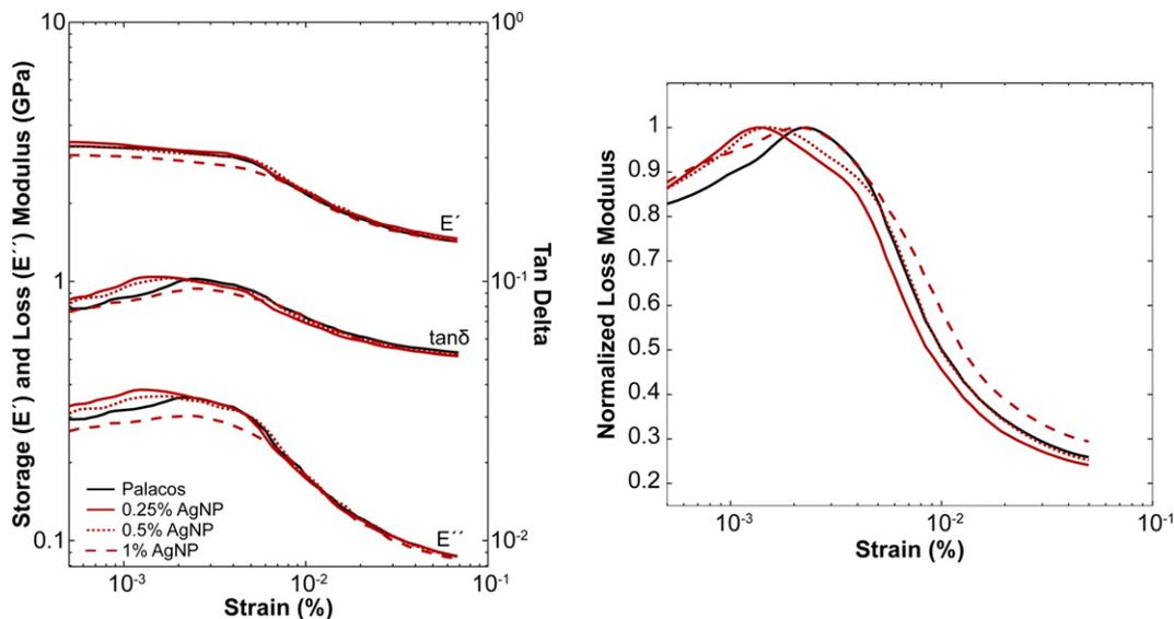
**Fig. 1.** Left — Results from DMA strain sweeps. Only data from 1 Hz is shown, for clarity purposes. At a loading frequency of 10 Hz, similar profiles for all cements were observed, however, the relative magnitudes were increased. Right — Normalized loss modulus curves ( $E''/E''_{\text{max}}$ ) for cements at a loading frequency of 1 Hz. The legend is applicable to both curves.
