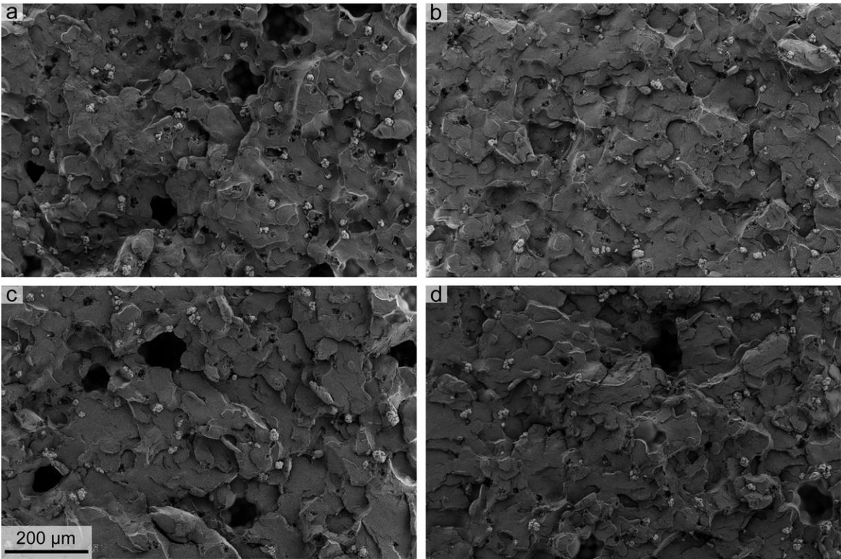
**Fig. 2.** Representative scanning electron micrographs at 300 $\times$  of the failure surface of four point bending samples. The scale bar is applicable to all images. a) Palacos, b) 0.25% AgNP, c) 0.5% AgNP, and d) 1% AgNP.
