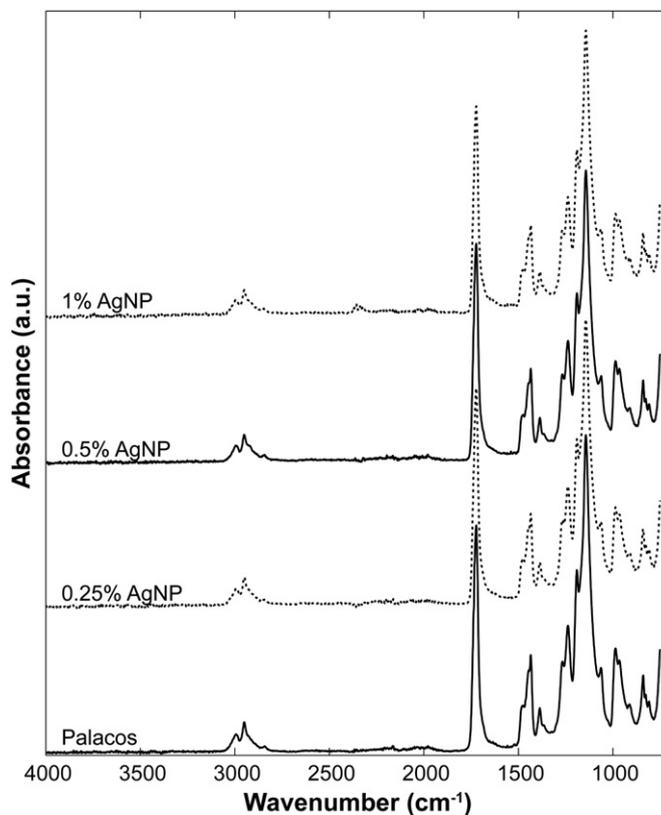
Fig. 4. Collected ATR-FTIR spectra for each cement. Each curve is an average of 96 individual measurements. The slight peak seen for 1% AgNP at  $\sim 2400\text{ cm}^{-1}$  is attributable to atmospheric  $\text{CO}_2$  and is not indicative of the material.
