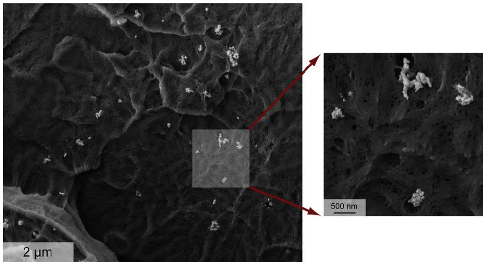
**Fig. 3.** SEM image taken at 10 kx (insert at 50 kx) showing small agglomerations of AgNPs.
