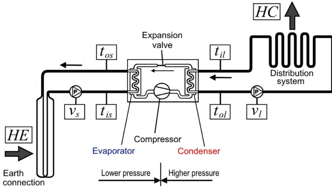
Fig. 1. Schematic diagram of GSHP in heating mode.
