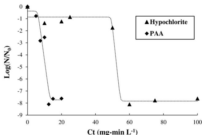
Fig. 1. Representative inactivation kinetics by PAA and hypochlorite for *E. coli*. pH = 7.5, log-linear fit model.
