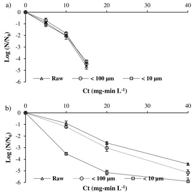
**Fig. 2.** Representative inactivation kinetics for total coliforms in primary effluent wastewater with different suspended solids size fractions using a) PAA and b) hypochlorite, pH = 7.5 (error bars ± 1 standard deviation,  $N = 4$ ).
