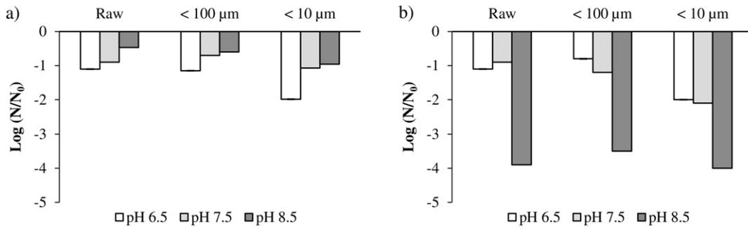
**Fig. 3.** Effect of pH on total coliform inactivation in primary effluent. a) PAA,  $Ct = 5 \text{ mg}\cdot\text{min L}^{-1}$  and, b) hypochlorite,  $Ct = 10 \text{ mg}\cdot\text{min L}^{-1}$  (error bars  $\pm 1$  standard deviation,  $N = 3$ , not visible on the scale).
