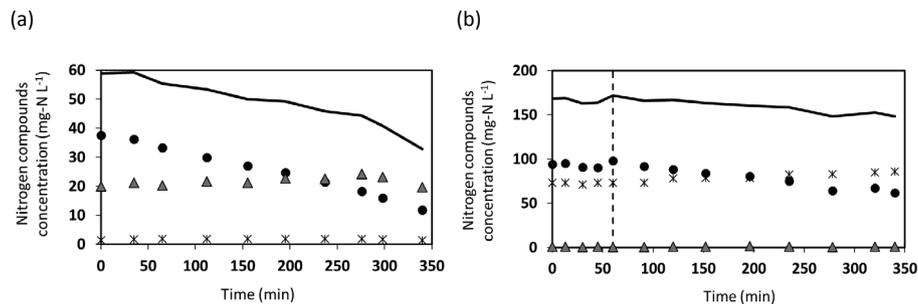
**Fig. 2.** Evolution of nitrogen compounds concentrations inside the reactor: TAN (●), NO<sub>2</sub>-N (\*), NO<sub>3</sub>-N (▲) and TN (—), for an operational cycle: (a) Stage A-II, day 74 and (b) Stage A-III, day 130.
