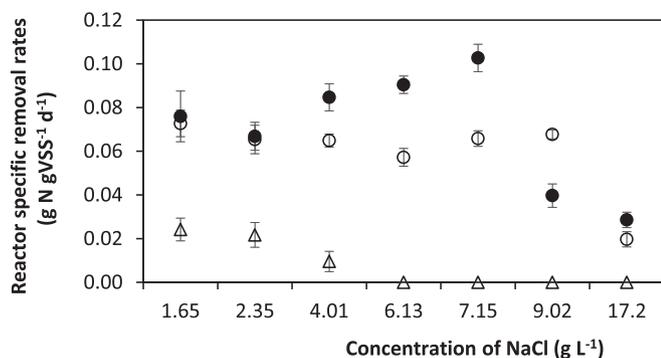
Fig. 3. Reactor specific removal rates for anammox (AR/X) (●), ammonia oxidizing (AOR/X) (○) and nitrite oxidizing (NOR/X) (△) bacteria obtained at different NaCl concentrations during the SBR operation. Specific rates were calculated by dividing removal rates by the biomass concentration inside the reactor (X,  $\text{g-VSS L}^{-1}$ ).
