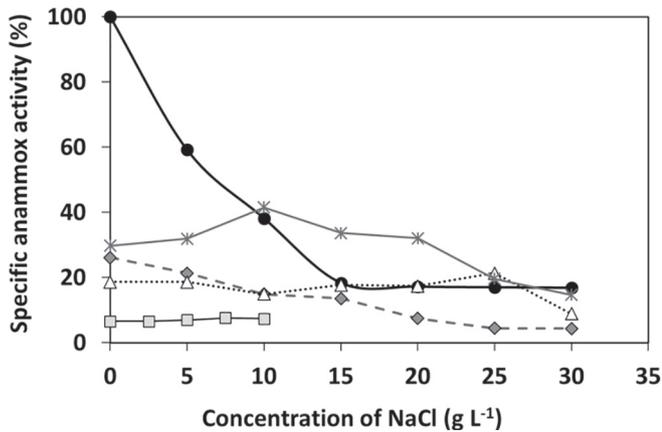
**Fig. 4.** Percentage of remaining SAA in the assays with the salt concentration for the SBR biomass on different operational days: inoculum (●), Stage A-IV on day 142 (■), Stage-B on days 11 (◆), 31 (△) and 39 (\*). The values correspond to average values of the experiments performed in triplicate (standard deviation lower than 10%).
