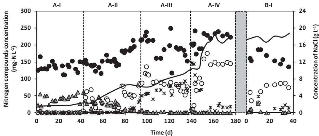
**Fig. 1.** Profiles of salt and nitrogen compounds concentrations in the different operational stages: NaCl (—), TAN in the influent (●) and TAN (○), NO<sub>2</sub>-N (\*) and NO<sub>3</sub>-N (▲) in the effluent.
