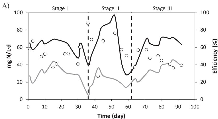
Fig. 1. (A) Evolution of the total nitrogen loading rate (mg N/(L.d)) in the influent (—) and effluent (---) and the percentage of total nitrogen removal efficiency (○). (B) Evolution of the nitrogen concentrations (mg N/L): total nitrogen in the influent (—) and ammonium (○), nitrite (●) and nitrate (▲) in the effluent.
