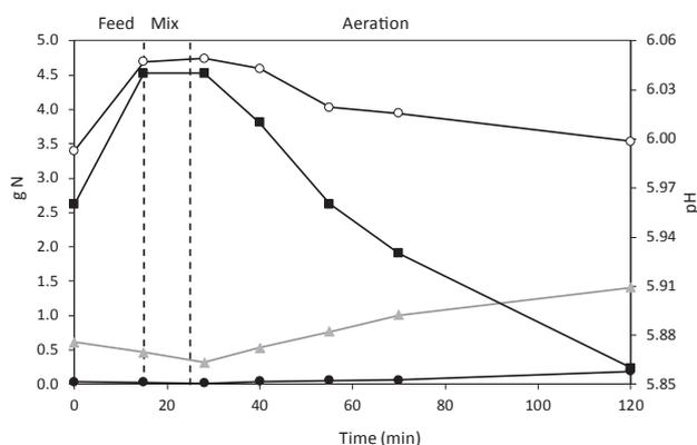
Fig. 3. Evolution of the nitrogen species during the SBR cycle with prolonged aeration (day 88): mass of ammonium (○), nitrite (●) and nitrate (▲) in g N, and pH (■).
