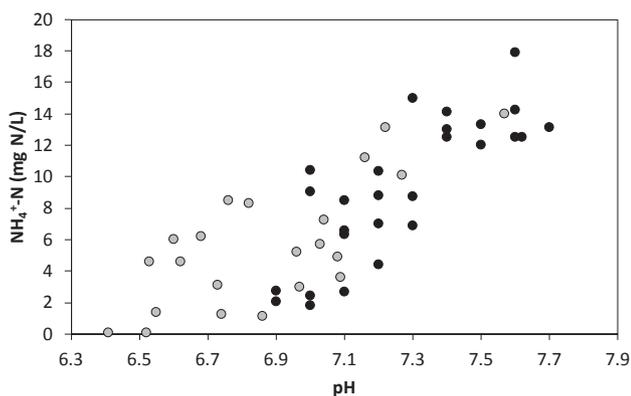
Fig. 2. Correlation between pH and ammonium concentration in the influent (●) and effluent (○) of the pilot SBR.
