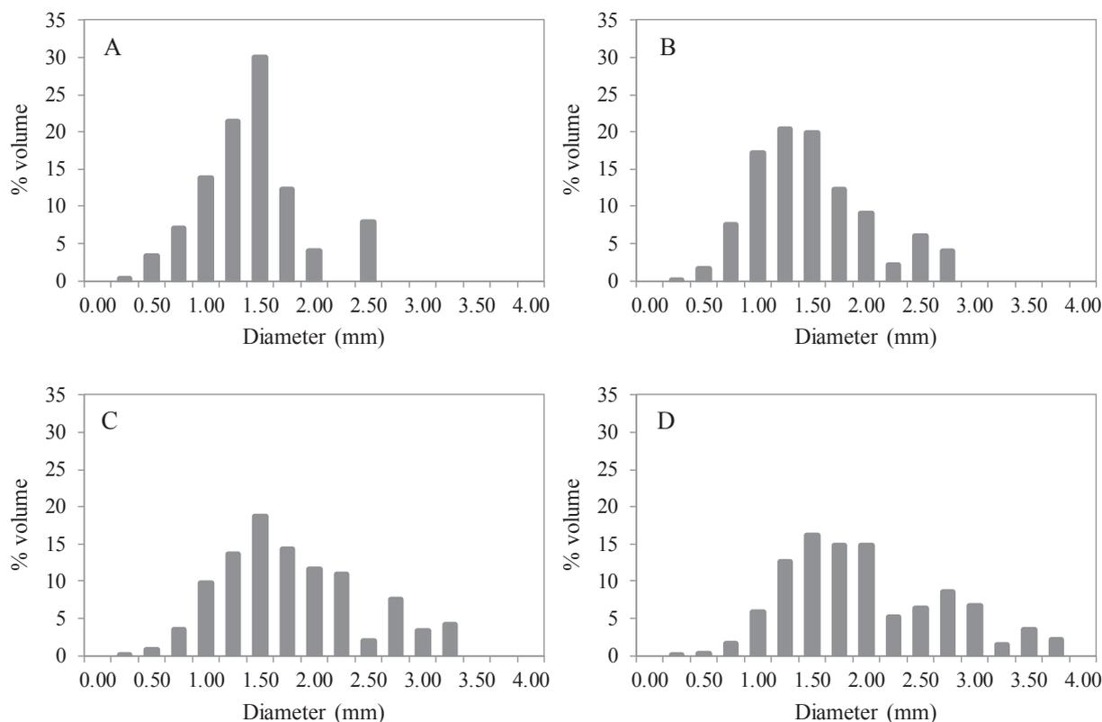
**Fig. 4.** Evolution of the volume distribution of the granules with respect to the average diameter on days 11 (A), 38 (B), 73 (C) and 93 (D).
