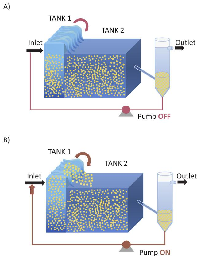
Fig. 1. Schematic system performance: A) recirculation pump stopped: biomass does not pass from tank 1 to tank 2, only liquid does; B) recirculation pump in operation: biomass passes from tank 1 to tank 2.
