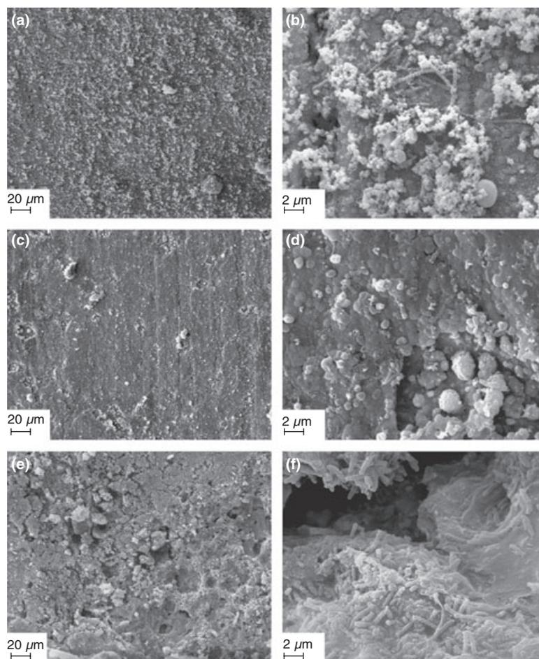
**Figure 4** SEM of the inner surface of copper pipes from the end point of corrosion tests and field samples. Representative images of copper pipes from biotic tests (a, b), abiotic tests (c, d), and field samples (e, f).
