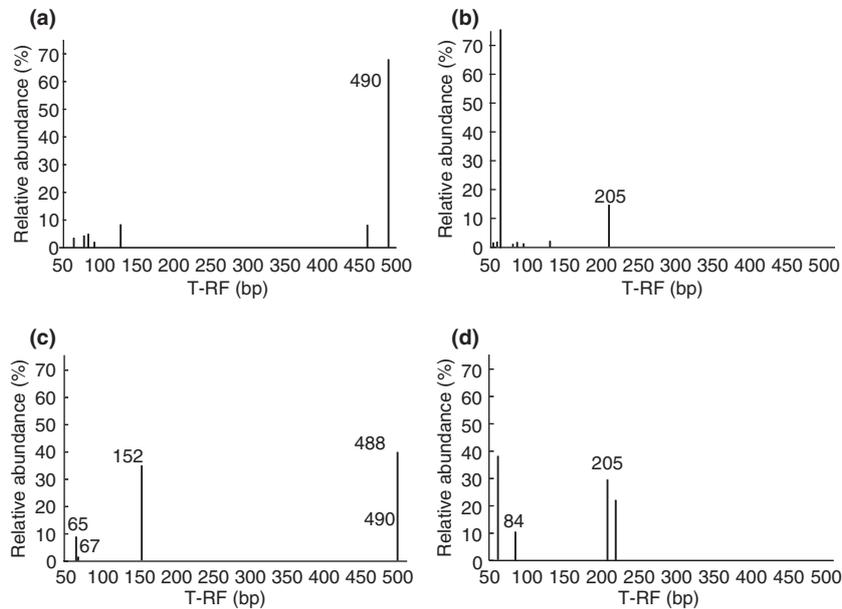
**Figure 5** Representative T-RFLP profiles of 16S rRNA gene sequences from copper pipe biofilm communities. Field samples T-RFLP profiles obtained with the *MspI* (a) or *HhaI* (b) endonuclease. Biotic tests T-RFLP profiles obtained with the *MspI* (c) or *HhaI* (d) endonuclease. The T-RF lengths that coincide with those determined for clone sequences are indicated.
