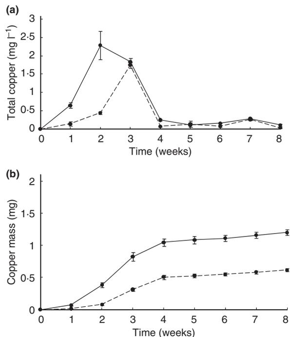
**Figure 2** Copper release from pipes in laboratory corrosion tests. (a) Total copper concentration. (b) Accumulated copper mass (solid line, biotic; dashed line, abiotic; mean ± 1 SD).
